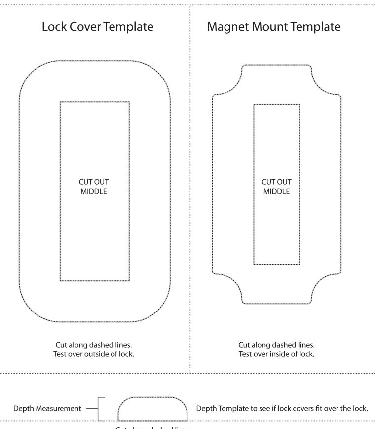
ATTENTION: This template is to test clearance around the lock cover and magnet mount for the GFC V2. It does not test for interference of the inside locking mechanism. PRINT AT 100%
